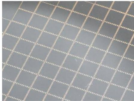
The appearance of **AuRoFUSE™** sealing frames (200 micrometers wide) printed on an 8-inch wafer
