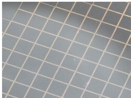
AuRoFUSE™ sealing frames (200 micrometers wide) printed on an 8-inch wafer
