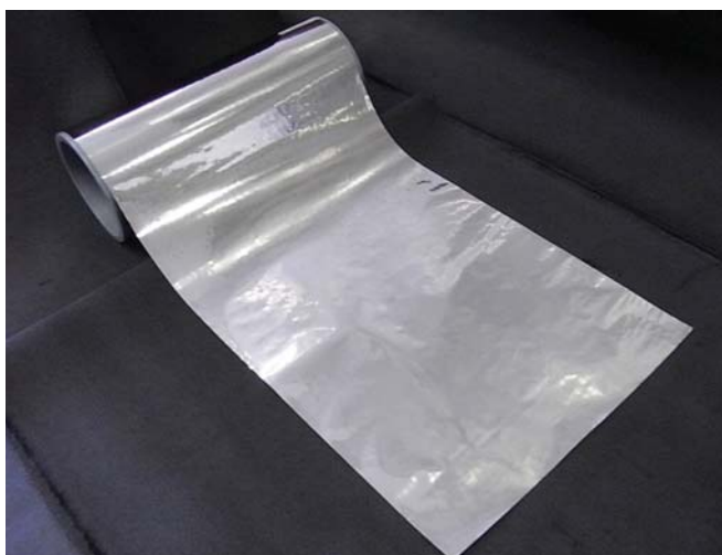
Fig. 4: Ultra-thin Pd-based alloy foil (5µm × 200mm)
