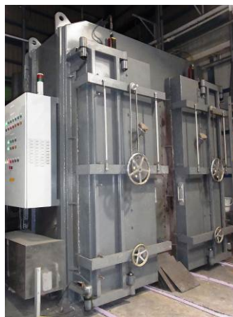
Furnace used for processing cyanogen compounds
