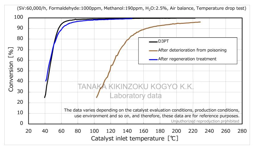
This is an example of catalyst poisoning by a silicon compound and regeneration of activity by our catalyst regeneration treatment.
