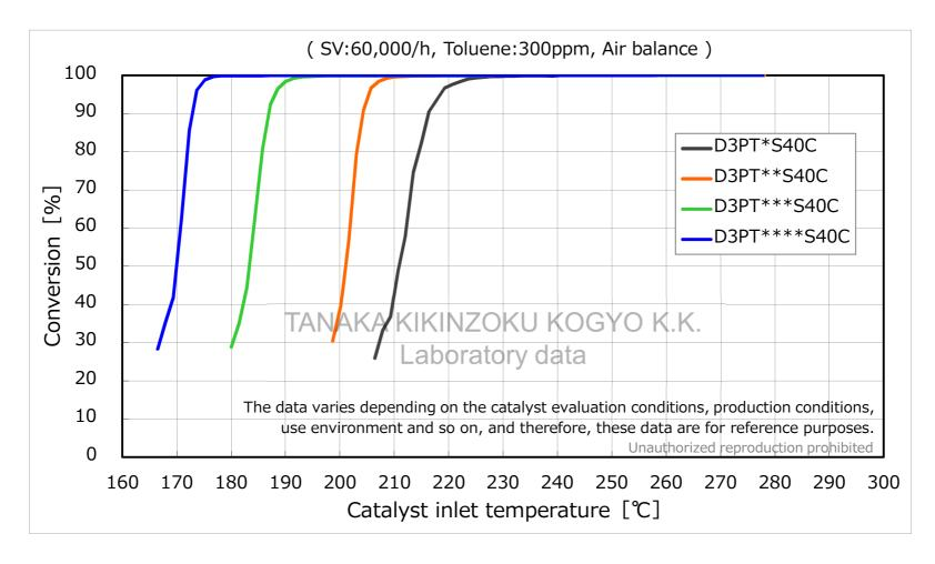
The amount of precious metal loading has a tremendous impact on the catalyst performance. We can propose low- loading products that differ from standard loading amounts to reduce costs as well as high- loading products to enhance performance.
